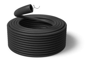
The PVC conduit with wire is ideal in standard installations that do not require the use of LSF0H materials; it is not suitable with liquid concrete and reinforced concrete. The conduit is made with ecological PVC and it is also internally lubricated. The colour of the conduit is black (RAL 9004).
