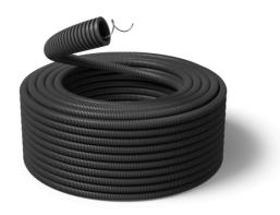
The PVC conduit with wire is ideal in standard installations that do not require the use of LSF0H materials; it is not suitable with liquid concrete and reinforced concrete. The conduit is made with ecological PVC and it is also internally lubricated. The colour of the conduit is black (RAL 9004).
