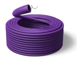
The PVC conduit with wire is ideal in standard installations that do not require the use of LSF0H materials; it is not suitable with liquid concrete and reinforced concrete. The conduit is made with ecological PVC and it is also internally lubricated. The colour of the conduit is violet (RAL 4008).
