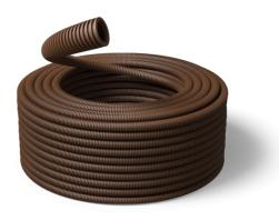
The PVC conduit is ideal in standard installations that do not require the use of LSF0H materials; it is not suitable with liquid concrete and reinforced concrete. The conduit is made with ecological PVC and it is also internally lubricated. The colour of the conduit is brown (RAL 8012).
