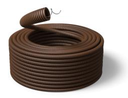
The PVC conduit with wire is ideal in standard installations that do not require the use of LSF0H materials; it is not suitable with liquid concrete and reinforced concrete. The conduit is made with ecological PVC and it is also internally lubricated. The colour of the conduit is brown (RAL 8012).
