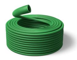
The PVC conduit is ideal in standard installations that do not require the use of LSF0H materials; it is not suitable with liquid concrete and reinforced concrete. The conduit is made with ecological PVC and it is also internally lubricated. The colour of the conduit is green (RAL 6037).
