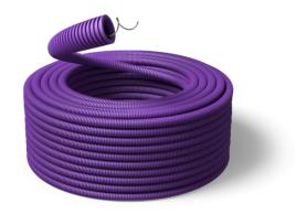
The PVC conduit with wire is ideal in standard installations that do not require the use of LSF0H materials; it is not suitable with liquid concrete and reinforced concrete. The conduit is made with ecological PVC and it is also internally lubricated. The colour of the conduit is violet (RAL 4008).
