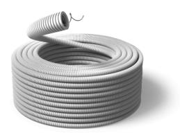
The PVC conduit with wire is ideal in standard installations that do not require the use of LSF0H materials; it is not suitable with liquid concrete and reinforced concrete. The conduit is made with ecological PVC and it is also internally lubricated. The colour of the conduit is white pearl (RAL 1013).
