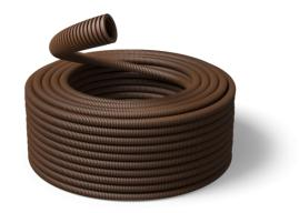
The PVC conduit is ideal in standard installations that do not require the use of LSF0H materials; it is not suitable with liquid concrete and reinforced concrete. The conduit is made with ecological PVC and it is also internally lubricated. The colour of the conduit is brown (RAL 8012).
