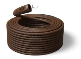
The PVC conduit with wire is ideal in standard installations that do not require the use of LSF0H materials; it is not suitable with liquid concrete and reinforced concrete. The conduit is made with ecological PVC and it is also internally lubricated. The colour of the conduit is brown (RAL 8012).
