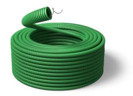
The PVC conduit with wire is ideal in standard installations that do not require the use of LSF0H materials; it is not suitable with liquid concrete and reinforced concrete. The conduit is made with ecological PVC and it is also internally lubricated. The colour of the conduit is green (RAL 6037).
