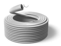
The PVC conduit with wire is ideal in standard installations that do not require the use of LSF0H materials; it is not suitable with liquid concrete and reinforced concrete. The conduit is made with ecological PVC and it is also internally lubricated. The colour of the conduit is white pearl (RAL 1013).
