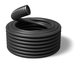
Double wall underground conduit, made in polyethylene, ideal for installation and protection of cables and electrical conduits in buildings and housing. Resistance to impact: 20J = IK10. Protection index: IP54, with couplings. Conduit smooth inside and corrugated outside.
