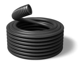
Double wall underground conduit, made in polyethylene, ideal for installation and protection of cables and electrical conduits in buildings and housing. Resistance to impact: 20J = IK10. Protection index: IP54, with couplings. Conduit smooth inside and corrugated outside.
