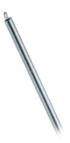
Bending spring made of steel and used for Halogen Free rigid pipes. At one end of the spring there is a loop that you should tie a longer and stronger thread to be able to pull it out more easily after you have bent the pipe.
