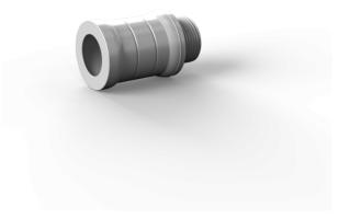
The tight couplings BK IP67 of PM SMART line, are used for the connection of rigid pipes with junction boxes. They are dust-tight and protected against the effects of temporary immersion in water, and they are also eco-friendly: Halogen Free according to European Standard EN 50642. Colour: grey (RAL 7035).
